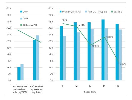
In 2019, the EXMAR Fully Pressurized fleet completed the second special survey dry dock. Maintenance works on the engines, hull and propeller performed during these technical stops, lead to a fuel efficiency increase as per following graphs.
