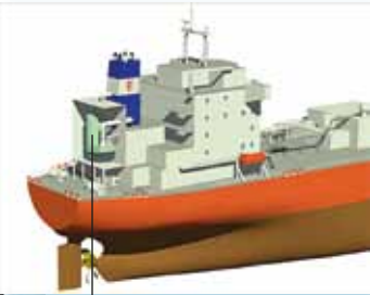
New funnel design with Scrubber to reduces Sulphur emissions
